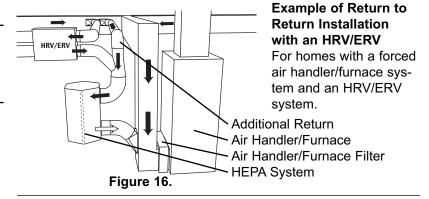
NOTE: This filtration system is an ADDITIONAL filter, and does NOT replace the existing air handler/furnace system filter.
